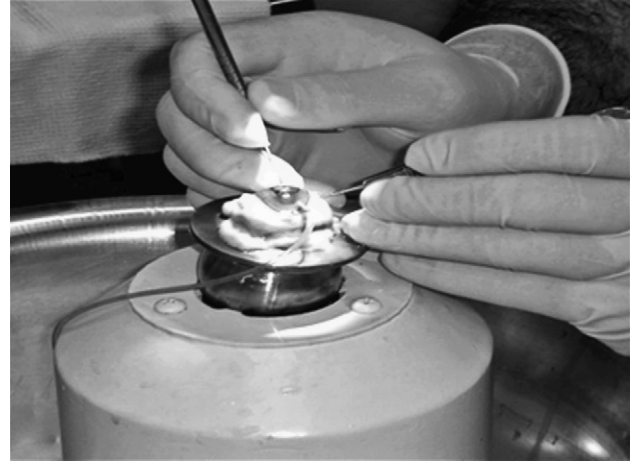
Figure 4. Surgical performance of the globe-fixation system on a mounted sheep eye. The upper portion of the base is designed to provide a convenient rest position for the surgeon’s hands.
